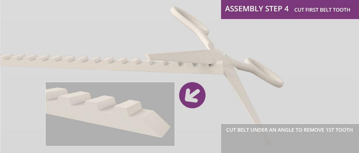
CUT BELT UNDER AN ANGLE TO REMOVE 1ST TOOTH
